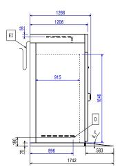
Electrical inlet (power) ΕI Refrigerant Outlet RO
